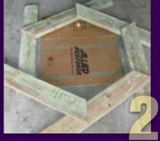
Lay the 6 boards around the cardboard "tree" to work out their length. Allow a space of 10-12cm between trunk and seat.
