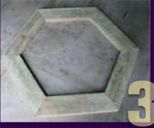
Mark a 30° angle on each board, and cut. Our tree diameter is 530mm, our cut boards measure 600mm on the longest edge.
