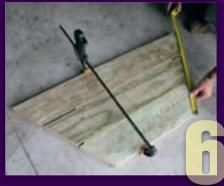
**Clamp boards**, with spacers, together. Measure the width at the edge. Cut 12 x braces, 20mm shorter than seat width.
