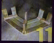
**Lay two sides** of your seat on ground upside down, with spacers in between. Stand legs on top, directly over joints.
