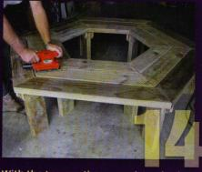
**With the two sections** complete, check that the remaining boards sit firmly in place. Don't fix yet. Sand and stain seat.
